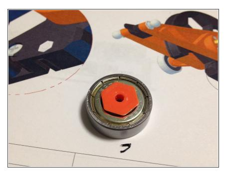
Insert 3d printed nut into ball bearing
