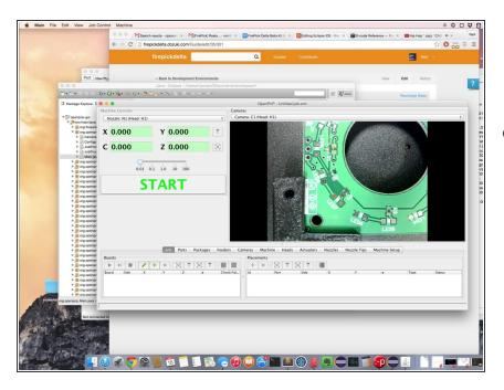
Now Start OpenPnP back up. If your camera and EMC02 motion controller are plugged in, you should see the camera image and be able to control your machine.
