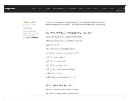
This guide will make heavy use of gcode (the protocol between the host software and the motion controller).
