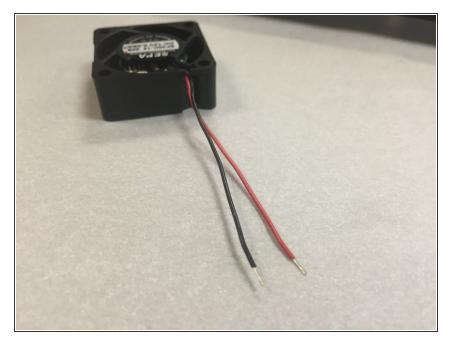
Strip the wires on the ends of both the fan and the cable.
