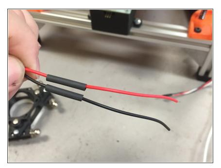
Add a ~20mm long piece of heat shrink tubing to each piece of wire.
