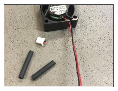
Cut the little connector off the end of the 30mm fan.
