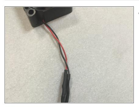
Shrink the heat shrink tubing with a heat gun.
