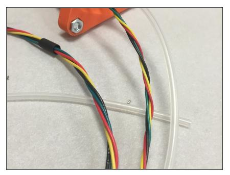
Wires should have been twisted when the modular tool / NEMA 8 motor assembly was being built. Ensure the wires are still tightly twisted.
