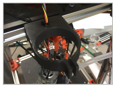
• Attach pump Mount to machine frame, using a M5 x 10mm buttonhead cap screw.
