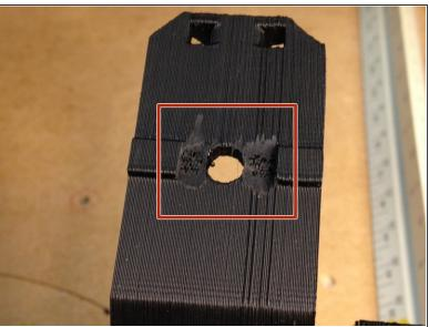
Trim the mounting bracket by removing a small portion of the ridge on the arm. See pictures.
