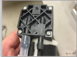
Connect the large tubing to the vacuum side of the pump.
