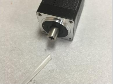
■ Insert the small tubing into the hollow shaft. Shove it down as far as it will go (~3-4 mm or so).
