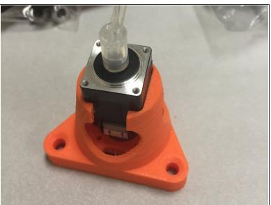
Add the epoxy to the gap between the large and small silicone tubes.
