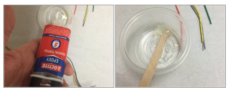
Mix up a bit of 2-part epoxy (not included in the kit). General purpose clear epoxy should work fine, this can be purchased from any hardware store, and even most big-box stores in the hardware section.
