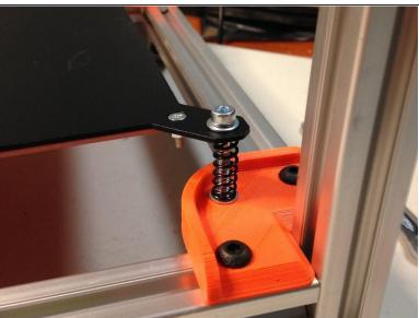
Ensure the screw heads are flat against the steel plate surface. Use your fingers to feel for any bumps.
