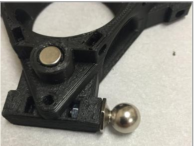
Insert the ball-studs into the ATC hub. Screw them down until they are tight, but not so much where the plastic deforms.
