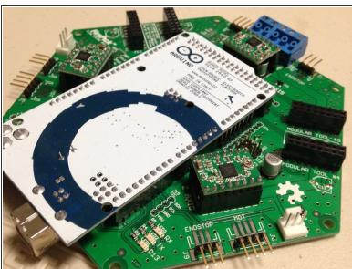
Insert Arduino onto EMC02
