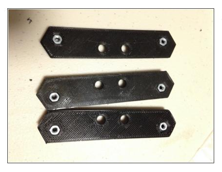
Insert M3 nuts into nut traps.
